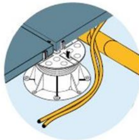
Concealing technical equipment
