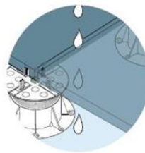
Presence of open joints avoiding all risks of cracking as compared to closed joints. Water evacuation made easier
